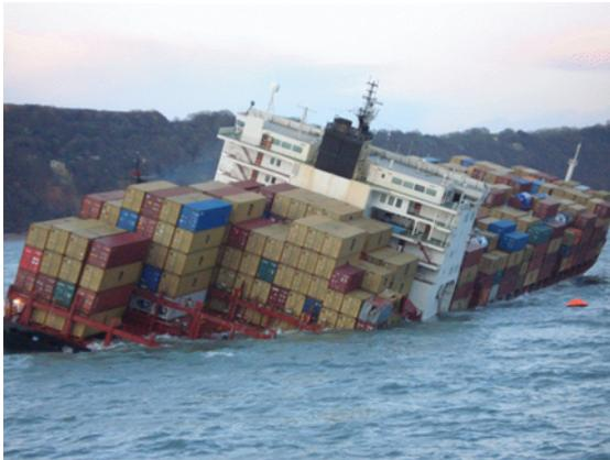
137 (20%) weighed more than 3 tons over their declared weights; the largest differential for a single container was 20 tons and the aggregate weight of the 137 containers was 312 tons more than shown on the cargo manifest!
